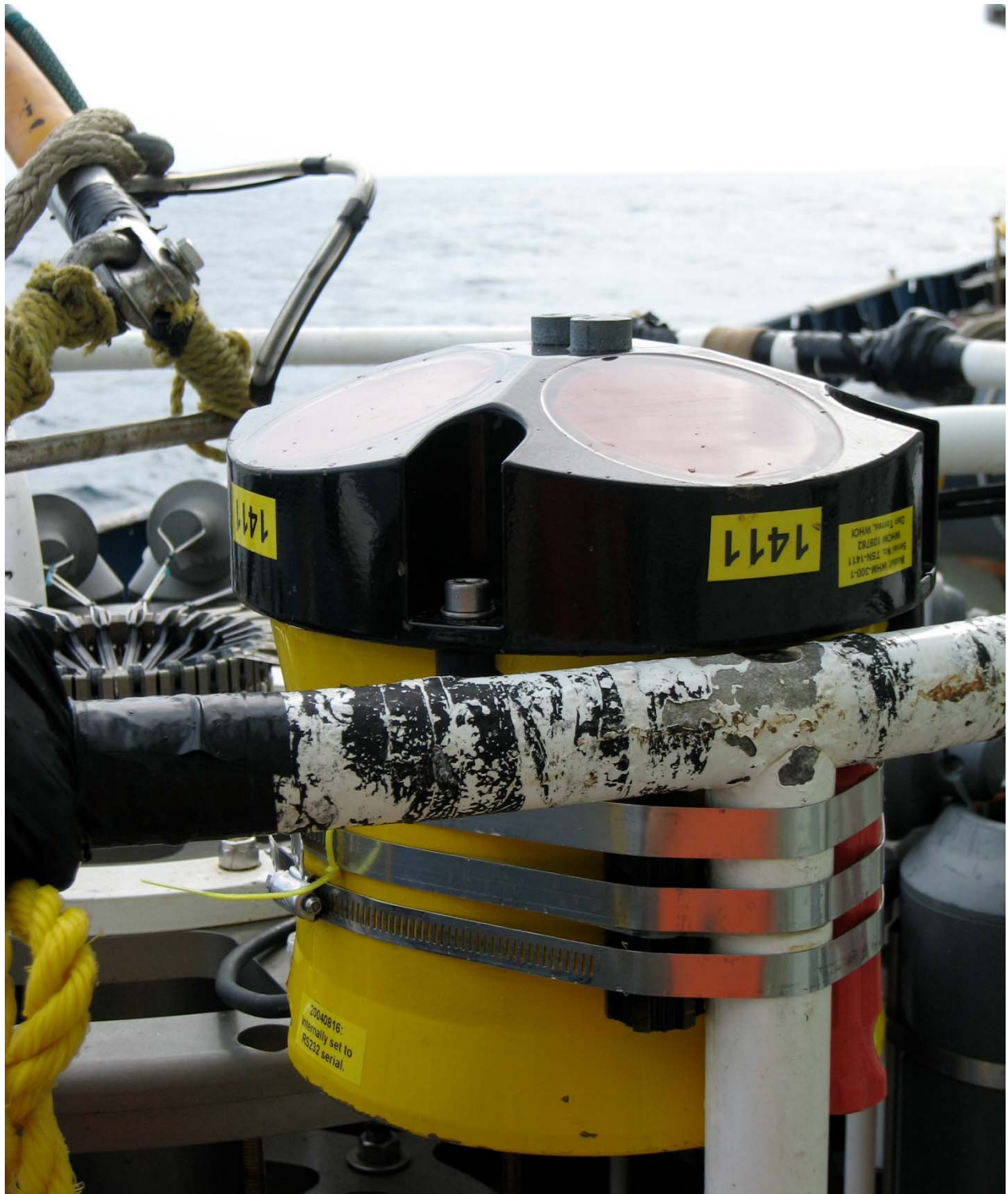
Figure 3. Teledyne/RDI Workhorse Sentinel installed as an uplooker using hoseclamps and screw-driver handles on a fully loaded CTD rosette.
