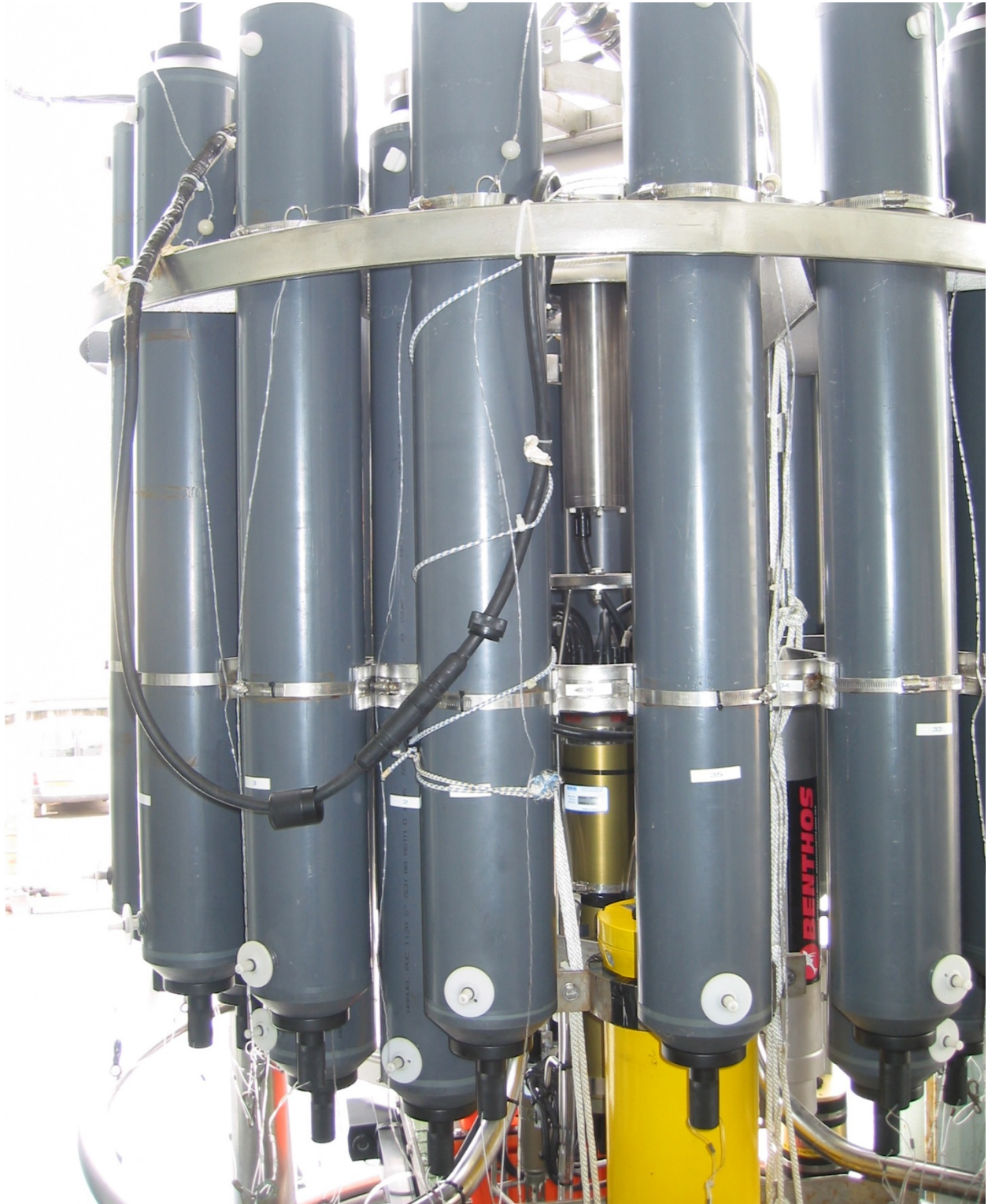
Figure 5. Octopus pigtail attached to a CTD sampling bottle with bungee cord. In this image, the pigtail is connected to the deck cable. When disconnected, the dummed-up lose end is tucked under the lower loop of bungee cord.
